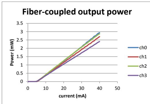
**Fig. 3a:** TOSA fiber coupled power.
