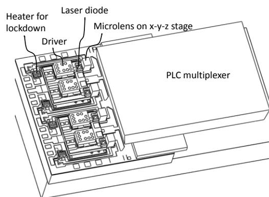
**Fig. 1:** 4x10Gb/s subassembly: The microlens is movable to optimize coupling from individual lasers to PLC
