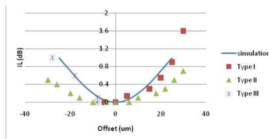
**Fig. 2a:** Additional loss as a function of error in x position between laser and PLC. Compensation with the lens allows loose initial positioning.
