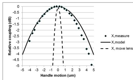
**Fig. 2b:** Additional loss as a function of solder shift at the heater. The dashed black line is calculated if the lens were to be locked down directly, showing high sensitivity, while the experimental points and the theoretical solid line shows the lower sensitivity of locking down the MEMS, with mechanical magnification.
