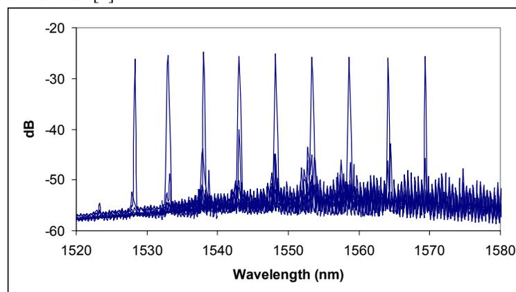
Fig. 3. Superimposed lasing spectra of the tunable laser
