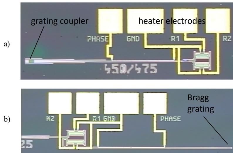
Fig. 1. The two variants of ring resonator reflector: a) loop mirror; b) with etched Bragg mirror.
