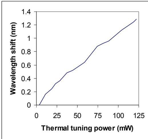
Fig. 4. Fine tuning of an individual lasing peak
