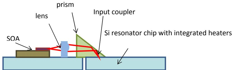
Fig. 2. Schematic diagram of tunable laser assembly with etched grating coupler on the reflector.
