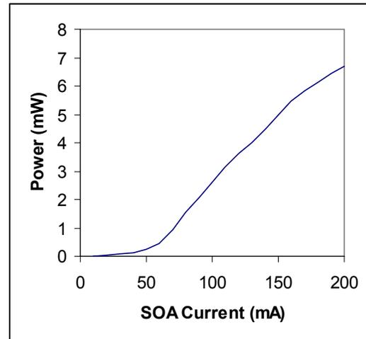
Fig. 5. Laser output power vs SOA current
